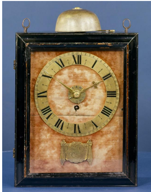
Salomon Coster (N5) Timepiece with alarm. Duration 30 hours. The only known Coster clock with alarm work.
